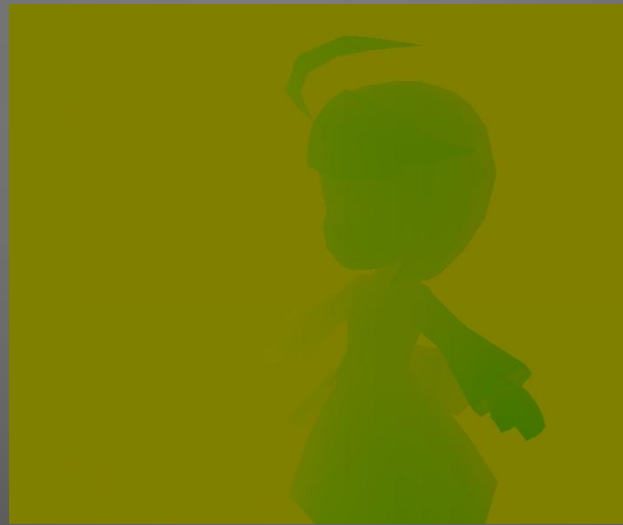
Screen Space Velocity Buffer with model rotating clockwise Normalized [0,1]
